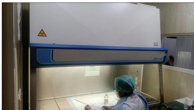
Figure 3: Biosafety hood with high-efficiency particulate air filter
